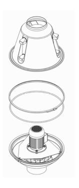
4. Mount round seal an upper part of housing on the lower part, fasten both housing halves together using the retaining ring
